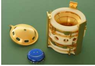
Fig. 2. The LEBIT high-precision Penning trap with the end-cap electrode removed.
